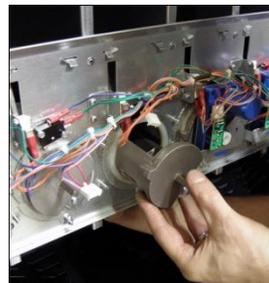
Insure that rear Auger Bushing does not become disengaged
